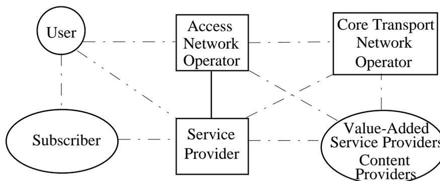
**Figure 1.** New Role Model and Service Delivery for UMTS
